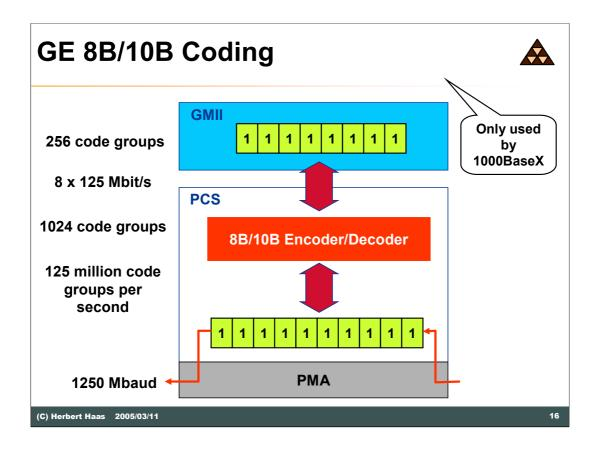
8B10B block coding is very similar to 4B5B block coding but allows fully balanced 10-bit codewords. Actually, there are not enough balanced 10-bit codewords available. Note that there are 256 8-bit codewords which need to be mapped on 1024 10-bit codewords. But instead of using a fully balanced 10-bit codeword for each 8-bit codeword, some 8-bit codewords are represented by two 10-bit codewords, which are sent in an alternating manner. That is, both associated 10-bit words are bit-complementary.
